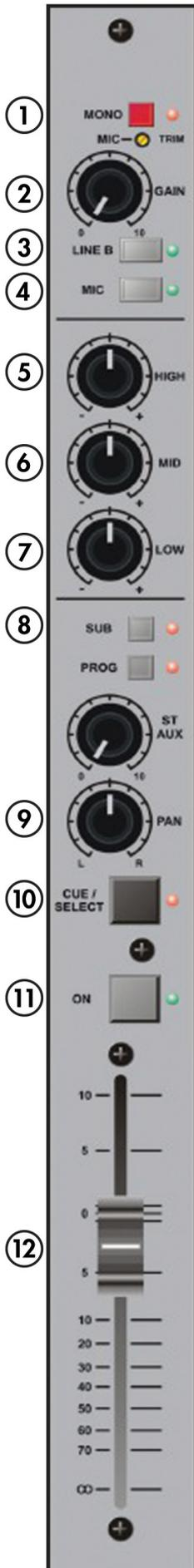
**1. MONO:** Enabling the Mono button turns a stereo signal into a mono signal. That means the same output is sent to both channels.
